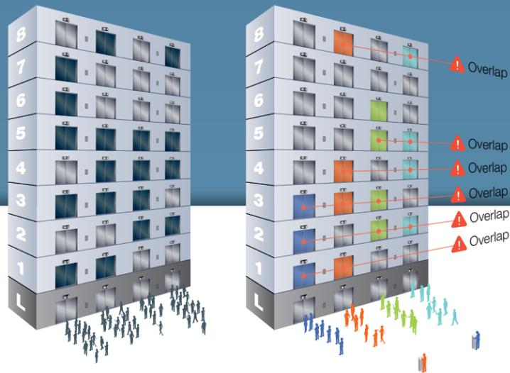
**Conventional up/down button systems** let passengers choose their own elevators. This results in disorganized travel paths. One elevator may stop at widely separated floors or multiple elevators might stop at the same floor.
