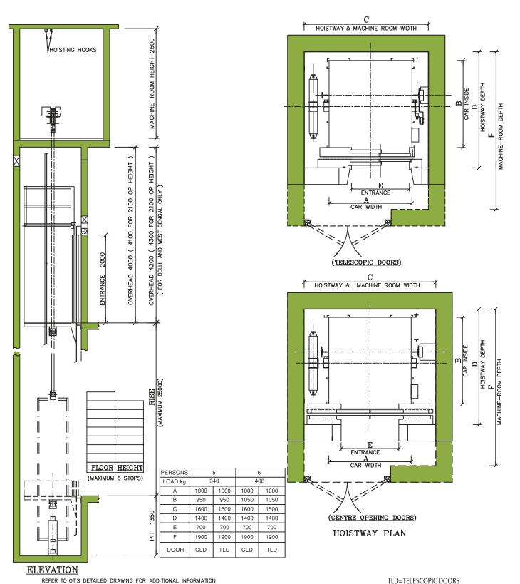
PM GEARLESS: (MACHINE-ROOMLESS) Speed: 0.7mps
