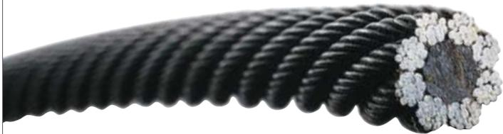
Otis Gen2 Mod's polyurethane-coated steel belts are stronger and more flexible, with a smaller bending radius allowing for a 70% smaller machine and increased durability and efficiency.
